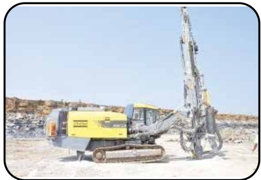
Drill with dust control system
