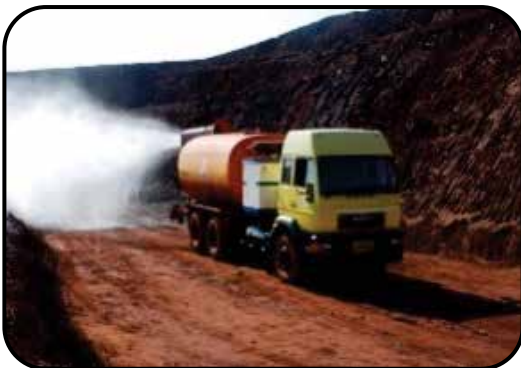
Mobile dry fog dust suppression system
