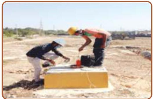
GW monitoring through piezometer
