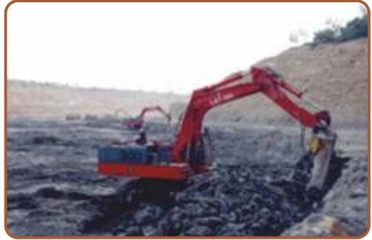
Rock breakers used for mining
